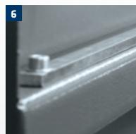
**1** The support surface for the rotary disk can be leveled; it is pre-adjusted to "0" in the factory.
